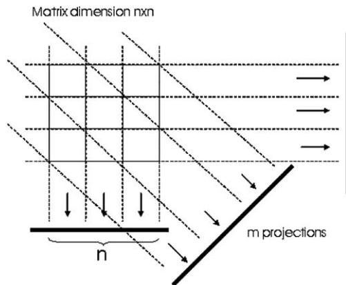
Fig. 2. Definition of the reconstruction procedure: The image (square matrix  $n \times n$ ) has to be reconstructed from the  $m$ -measured projections, each one with length  $n$ .
