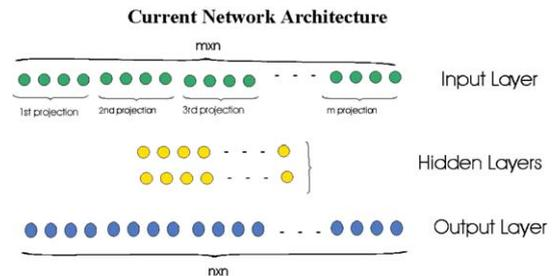
Fig. 3. Network Architecture: The Input Layer comprises  $m \times n$  nodes supplied with the projection data. The reconstructed image ( $n \times n$ ) is represented by the Output Layer.
