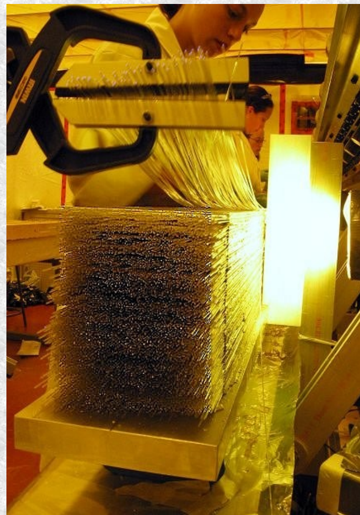
Students construct a prototype BCAL module in Edmonton, Alberta.
